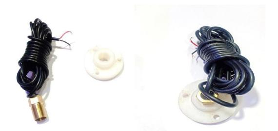
SPECIFICATION: **Material:** Brass **Threads :**1.5 BSP **Día :**47.8mm **Length:** 70mm **Hex :**50mm **Sensing Range:** 3 max. Meter distance **Sensor cable:** 3 meters
